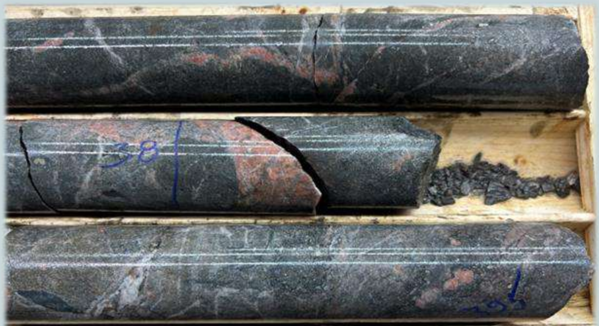
Carbonatized lamprophyre and vein syenite. Scarce pyrite
