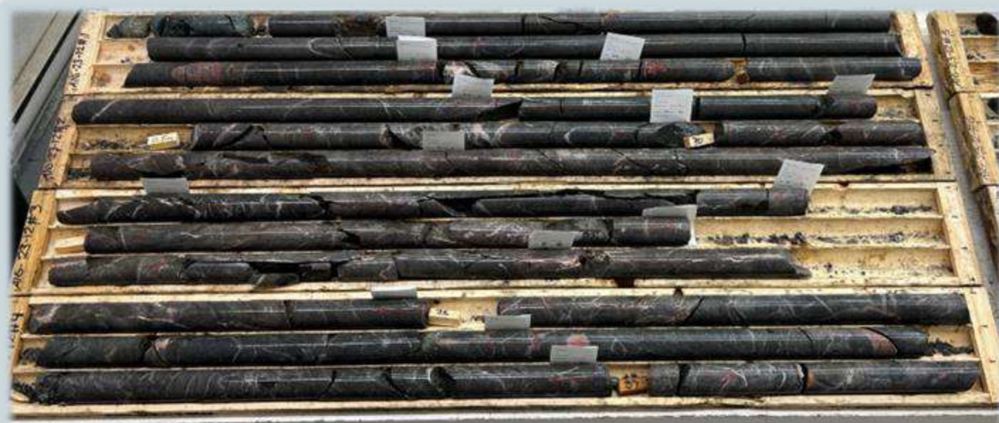
Carbonatized lamprophyre and vein syenite. Scarce pyrite
