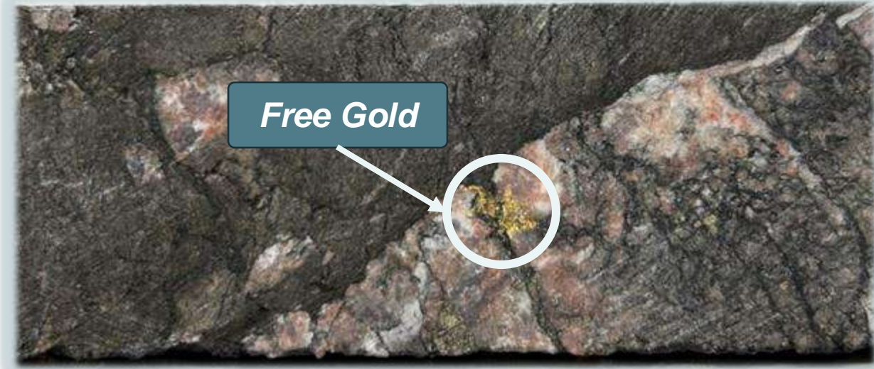
Carbonatized lamprophyre and vein syenite. Scarce pyrite
